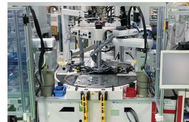
Production facilities for automotive connectors using SCARA robots
